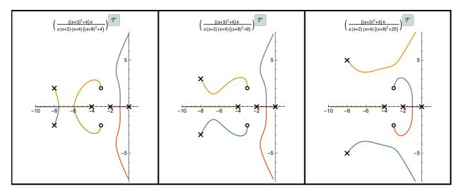
We can have break-away points that are not on the real axis. You can also have a single break-away point where more than two poles meet. These are typically pathological scenarios; if we nudge any of the poles in any direction, we obtain a more typical-looking locus. Examples below.
